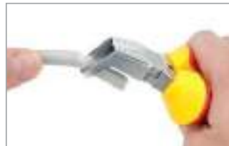
Bend the cable end slightly until the separation point breaks, and pull off the piece of sheath
