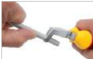
Carefully cut into the sheath with the blades until the stop rests against the sheath. Then rotate the pliers part way around the cable
