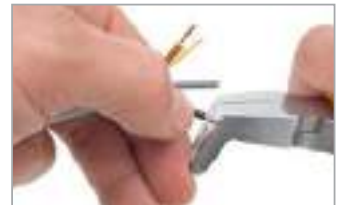
Remove the insulation of the individual conductors with the stripping holes
