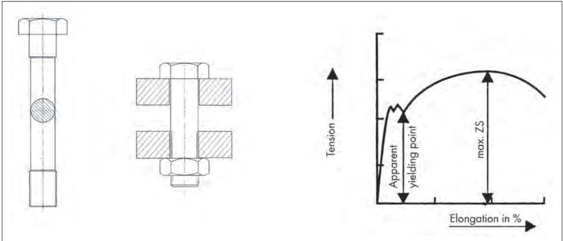
Tensile test on a turned-off screw
